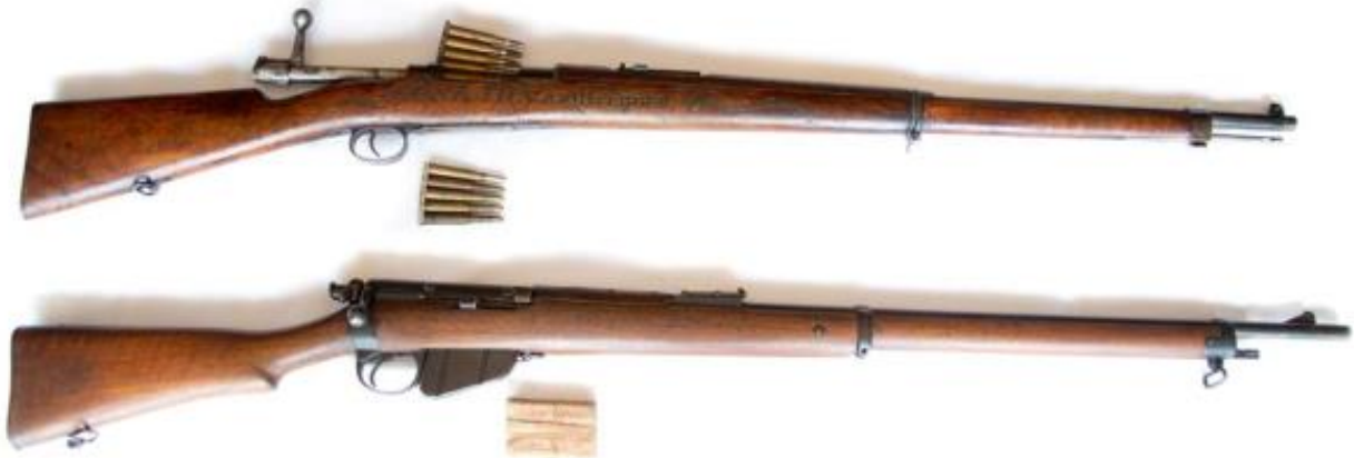
Boer Mauser with clips holding five Mauser cartridges (top) and Lee-Enfield (bottom) with paper wrapped package holding ten loose rounds.
